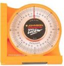
Lay a level or piece of wood on the stairs, sit the angle finder on the wood and just read off the slope. Check a couple spots ie top middle bottom. Most stairs run somewhere around 33 - 36 degrees.
